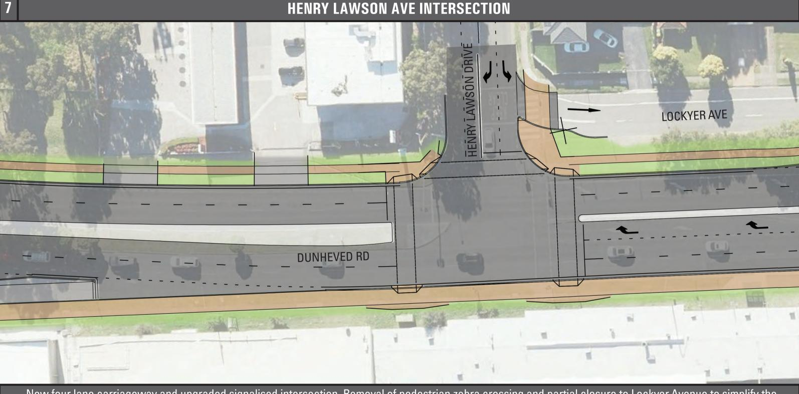
New four lane carriageway and upgraded signalised intersection. Removal of pedestrian zebra crossing and partial closure to Lockyer Avenue to simplify the intersection. Vehicles will now exit Lockyer Avenue at John Batman Avenue.
