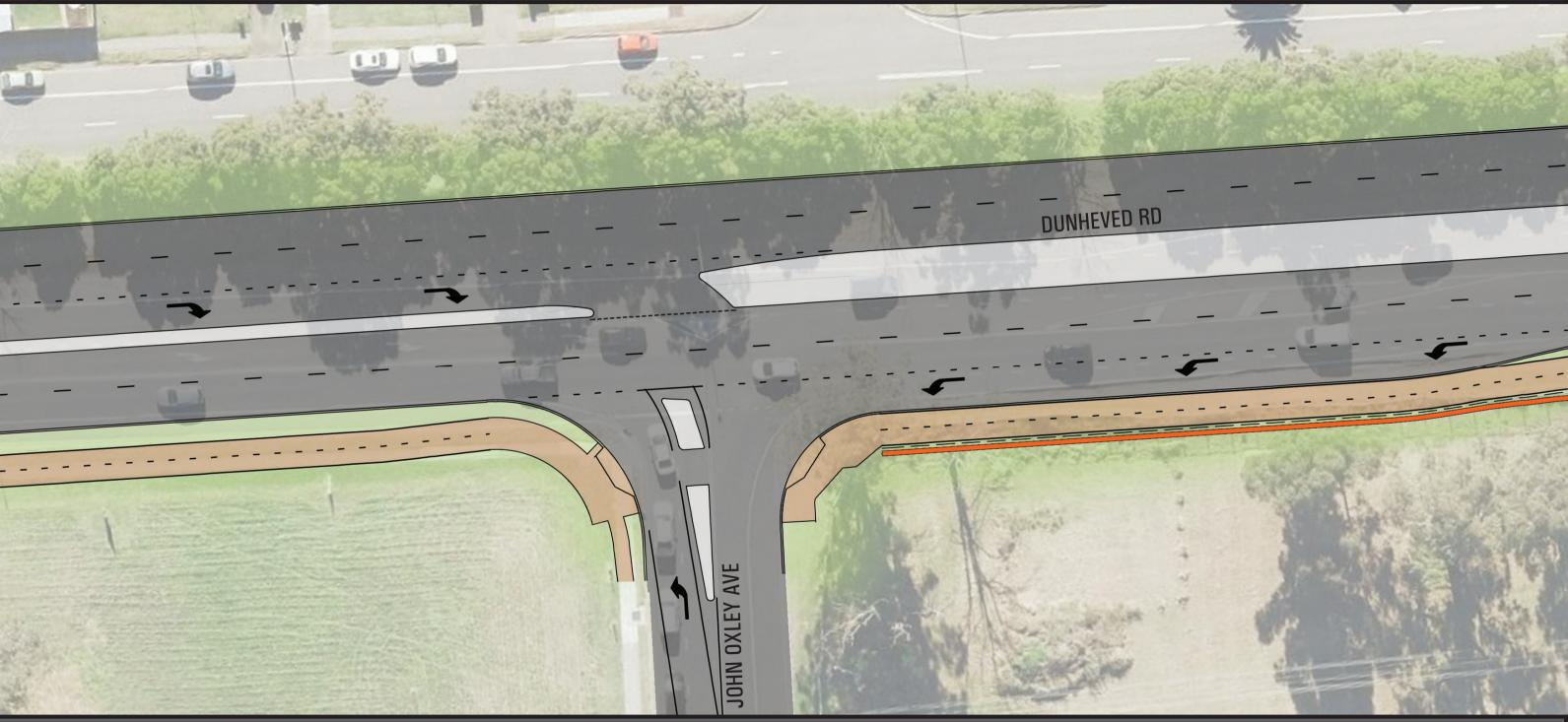
New four lane carriageway and upgraded intersection. Upgraded intersection with right turn permitted into John Oxley Avenue and the current westbound left in / left out access maintained for John Oxley Avenue. Safer eastbound access to Dunheved Road from Werrington will be via upgrade traffic signals at Francis Street or via the Parks Avenue and Werrington Road intersection.
