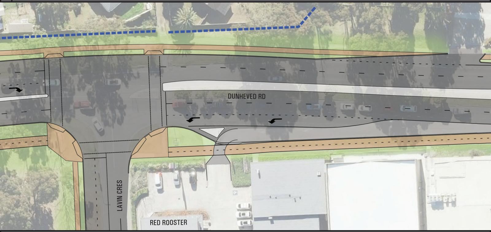
New four lane carriageway, new signalised intersection and maintain left lane into shopping area with a 400mm wide median separator
