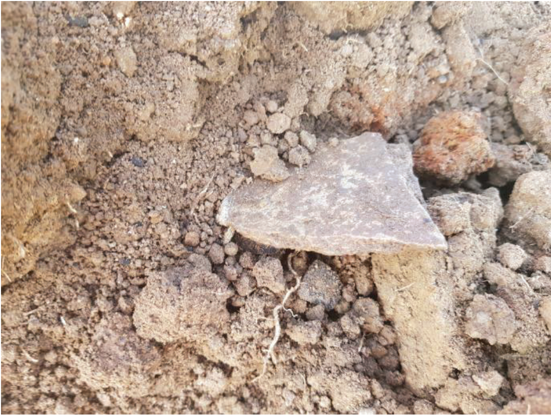
Image 11.1.3 View of ACM encountered at TP21 at 0.3m bgl
