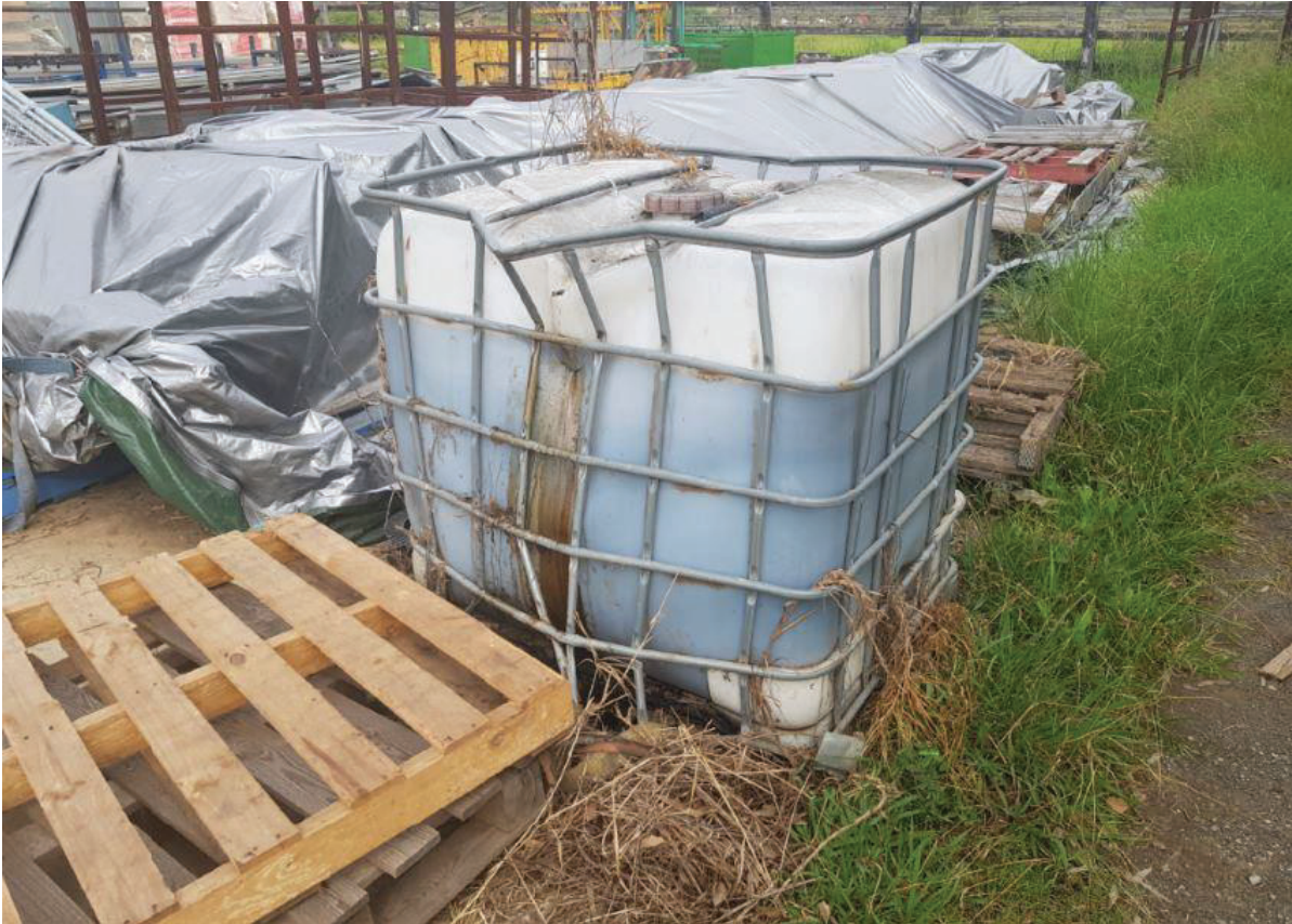
Image 6.5.1 View of oil stored in IBC, with slight leak
