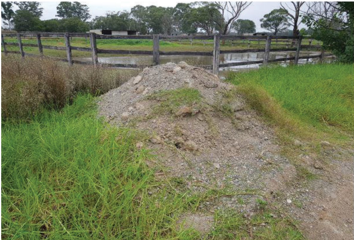
Image 6.10.6 View of stockpile (SP4) containing silt and aggregate with demolition waste inclusions
