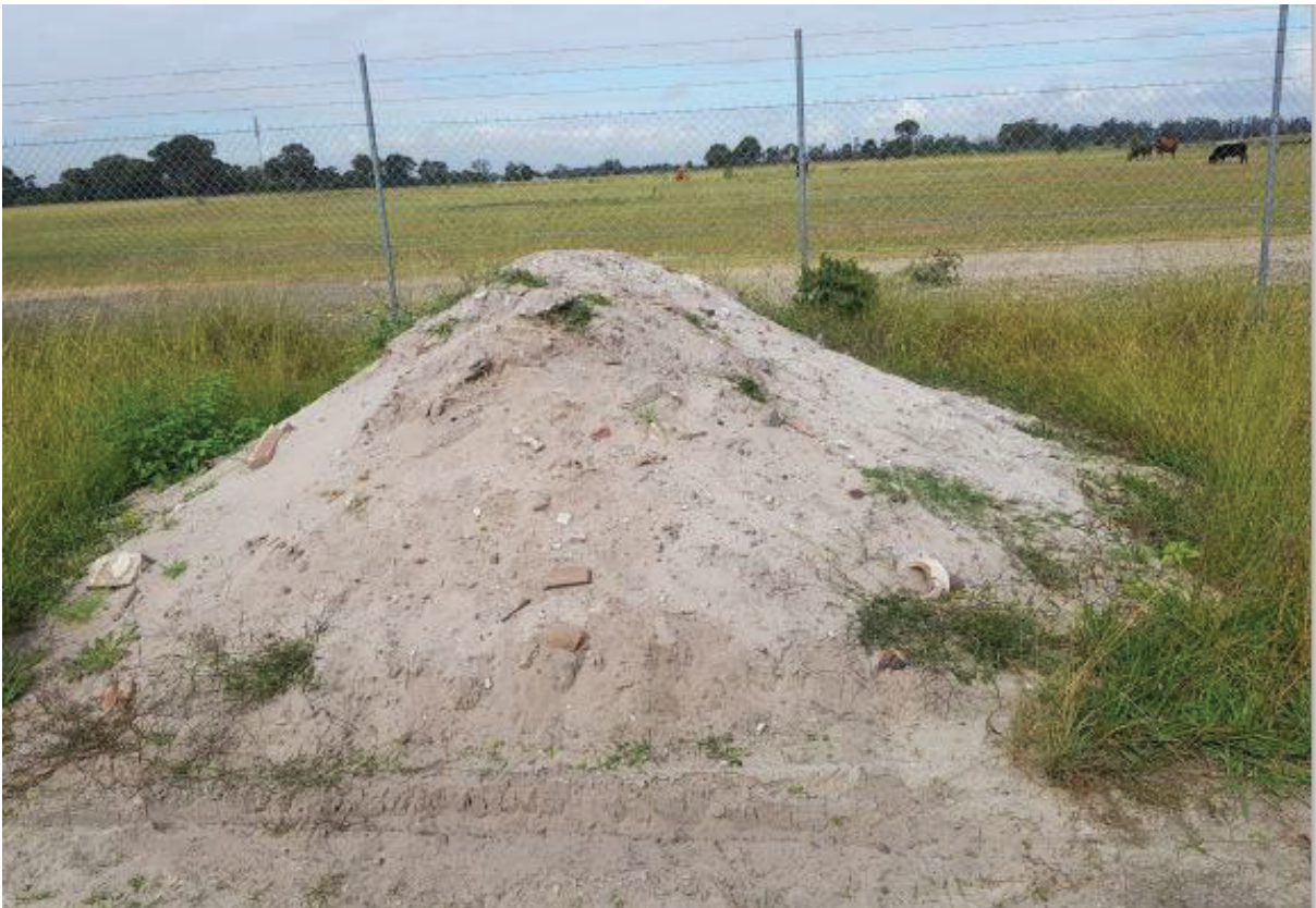
Image 6.10.4 View of sand stockpile with demolition waste inclusions (SP1)
