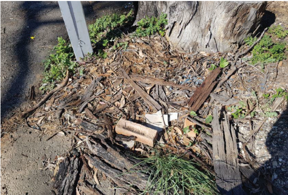
Image 6.9.2 View of potential asbestos containing fibrous cement sheeting
