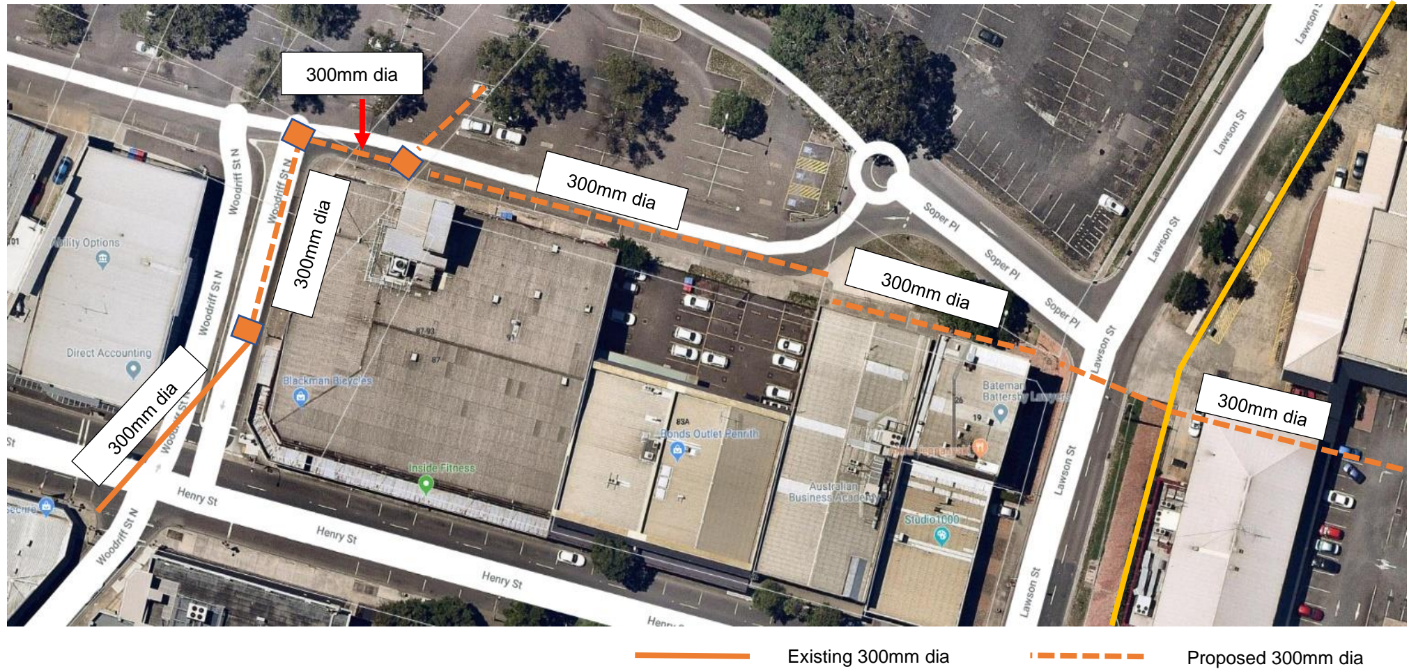
Figure 8 - Sewer alignment for new 300mm dia main (Nearmap, 2019)
