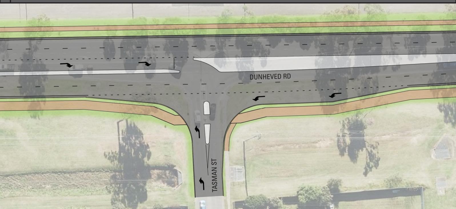
New four lane carriageway and upgraded intersection. Upgraded intersection with right turn permitted into Tasman Street and the current westbound left in/left out access maintained for Tasman Street. Safer eastbound access to Dunheved Road from Cambridge Park will now be via the upgraded traffic signals at Francis Street.
